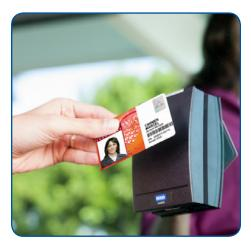
iCLASS SE readers include Open Supervised Device Protocol (OSDP), a new Security Industry Association (SIA) standard that together with Secure Channel Protocol (SCP) provides secure communications and central management.
